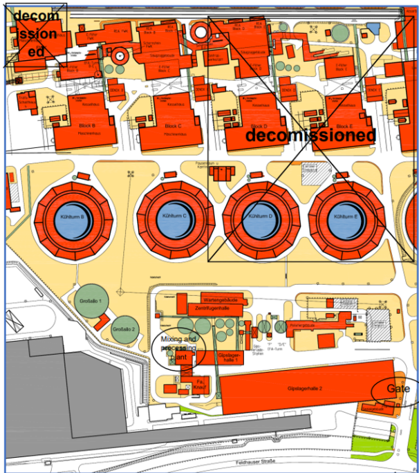
Figure 2. Layout of power plant Scholven
